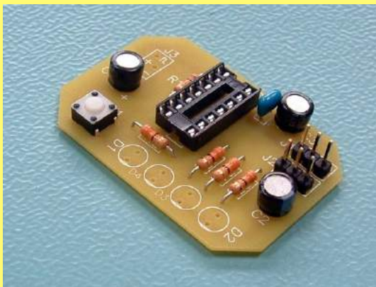
PICTURE 5: Add tactile switch (button)
