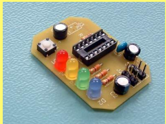
PICTURE 6: Fit 4 x LEDs as shown
