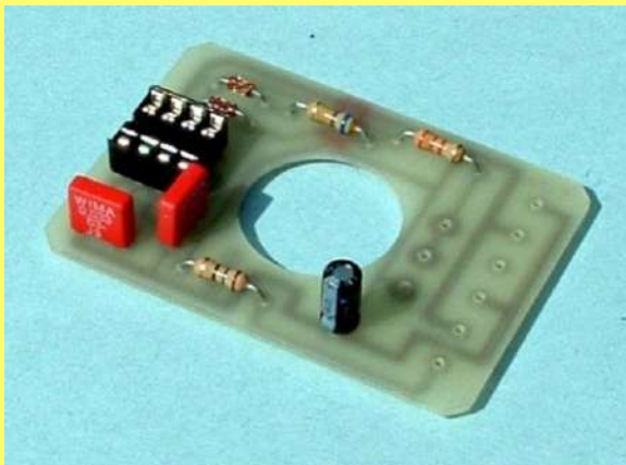
Picture 3: Capacitors added
