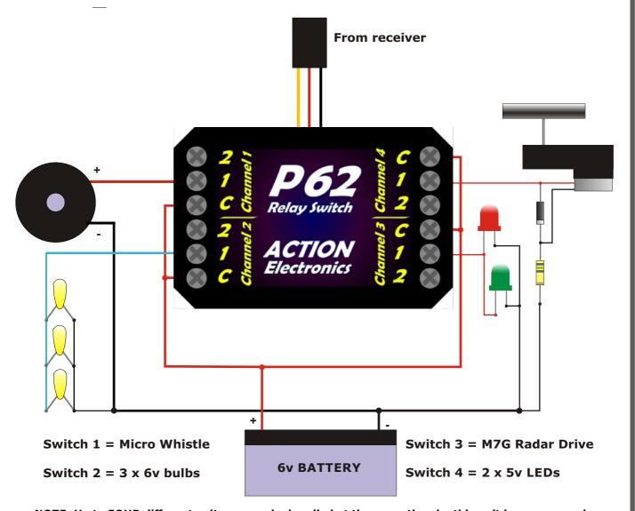
NOTE: Up to FOUR different voltages can be handled at the same time by this unit i.e. one per relay.
