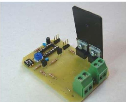
**PICTURE 7: TB2 and first pair of MOSFETs with heat-sink tab fitted**
