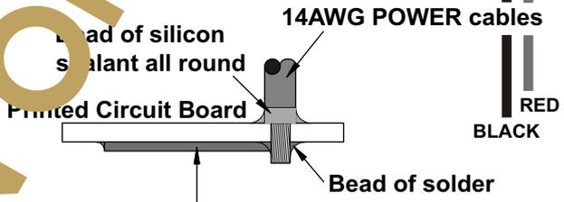
Solder 13mm piece of copper wire to copper land as shown. Use a good bead of solder!
