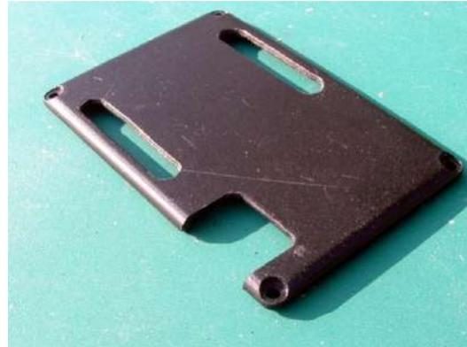
**PICTURE 12:** Remove masking tape and clean up filed edges with a fine file or scrape smooth with a sharp knife-blade.
