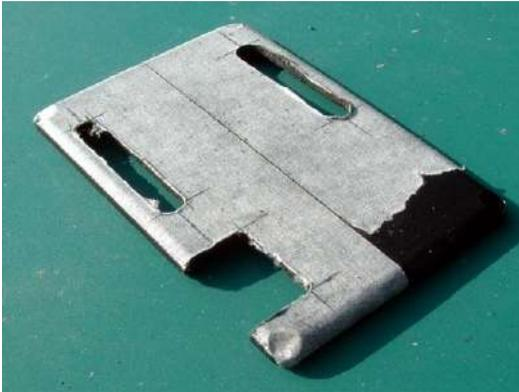
**PICTURE 11:** Snip between webs with side-cutters; push out surplus ABS. Use warding files to file back shape to pencil outlines.
