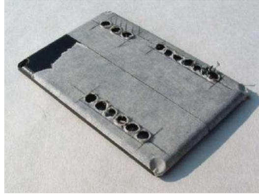
**PICTURE 10:** Drill a series of holes within outline of cut-outs
