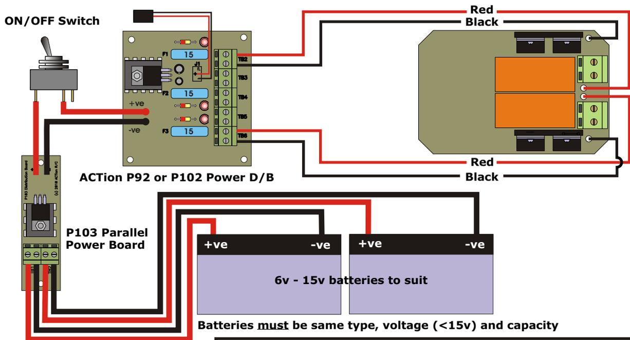
**FIG #6: TWO BATTERIES CONNECTED IN PARALLEL**
