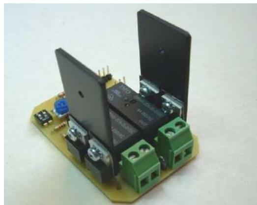
**PICTURE 8: Relays & second pair of MOSFETs with heat-sink tab fitted**
