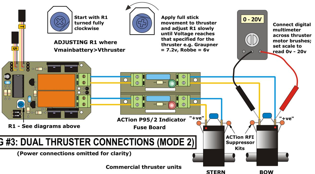
**FIG #3: DUAL THRUSTER CONNECTIONS (MODE 2)**
