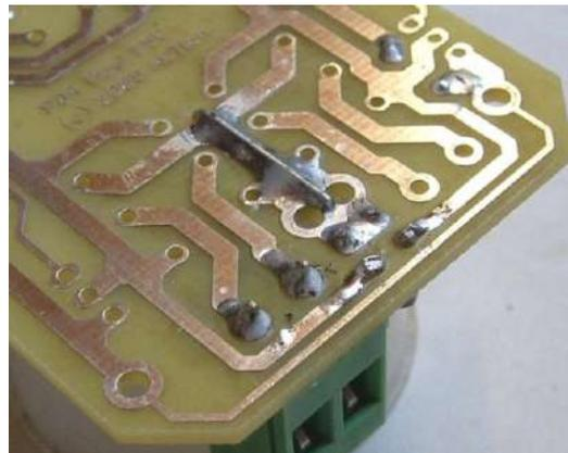
**PICTURE 6: Close-up of reverse of PCB showing copper wire shunt**
