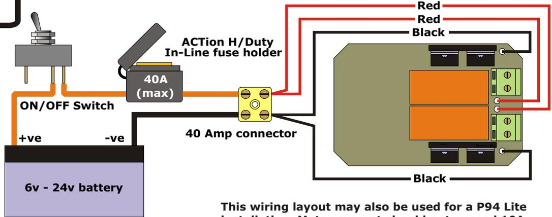
This wiring layout may also be used for a P94 Lite installation. Motor current should not exceed 10A each and a 20A fuse (max) should be used.
