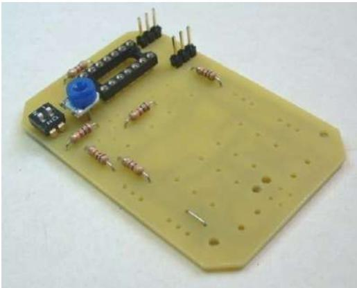
**PICTURE 3: Resistors & wire link**
