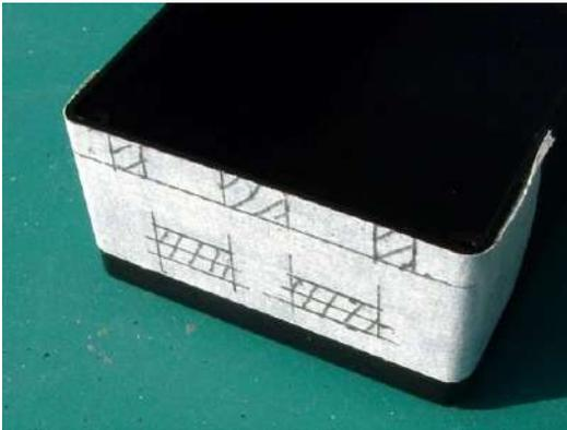
**PICTURE 13:** Tape and mark out holes for cables in end of case
