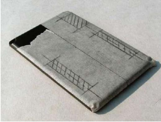
**PICTURE 9:** Cover lid with masking tape and mark cut-outs with sharp pencil
