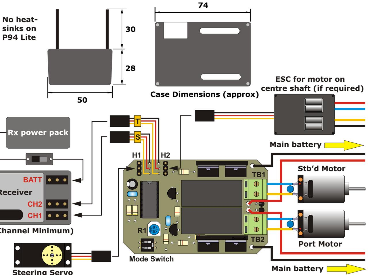
**SCHEMATIC OF INSTALLATION IN TWIN-ENGINE MODEL**
