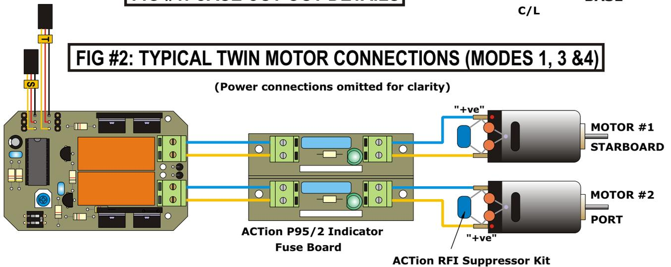
When connected as shown, the LEDs will both glow the same colour when the main drive motors rotate in opposite direction e.g. At Full Ahead speed. Adjust rudder trim lever of transmitter until the two LEDs "fire up" together when slight forward throttle command is given (does not apply to Mode 1).
