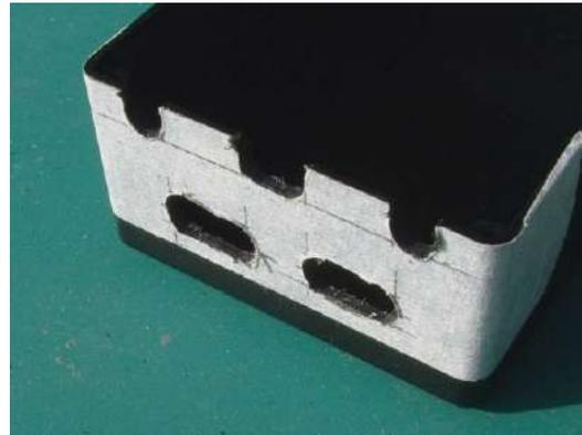
**PICTURE 14:** Drill and file back to pencil outlines; clean up edges as shown
