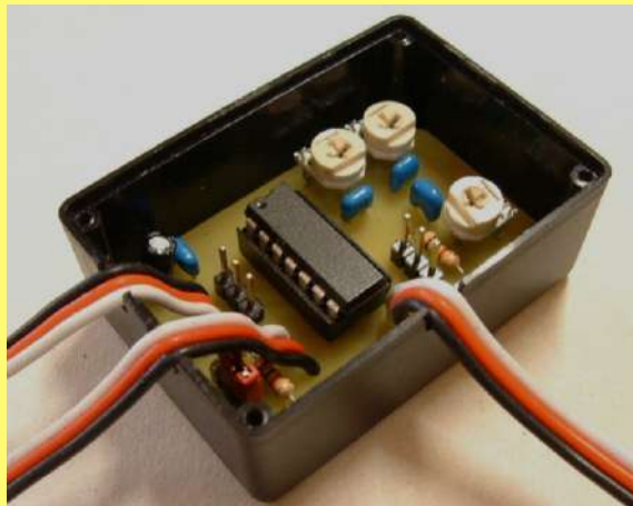
PICTURE 5: Fit PIC chip. NOTE! ANTI-STATIC PRECAUTIONS REQUIRED
