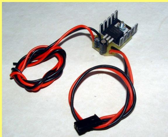
Picture 6- Finished unit with input lead fitted.
